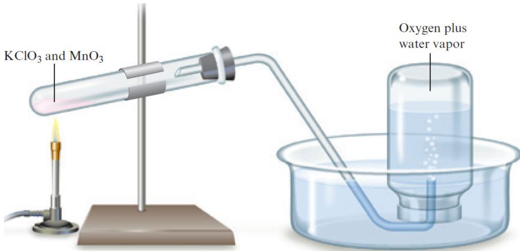
Figure 5.13 - The Production of Oxygen by Thermal Decomposition of Potassium Chlorate
