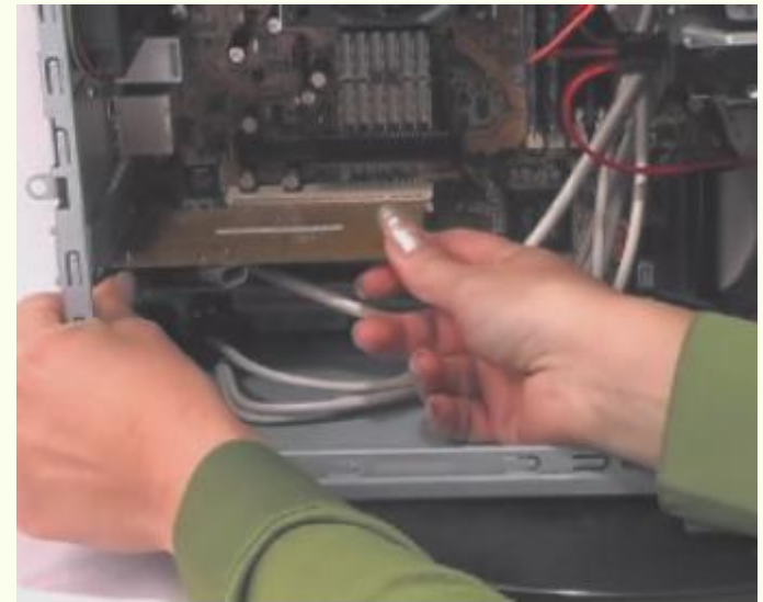
Figure B-29: An expansion card slides into an expansion slot
